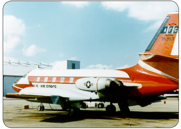
FLIGHT CHECK AIRCRAFT: A C-140A "Jet Star" aircraft is painted in the bright orange and white scheme of an Air Force Communications Service flight check aircraft.
