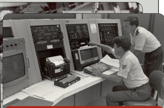
An AFSATCOM programmer, Tech. Sgt. Otis Smith, operates the AFSATCOM simulator while 2nd Lt. Rick Mahoney, Test Analyst watches. The simulator was capable of reproducing the necessary inputs and outputs that show real-world choices that can be handled by radio receiver, transmitter, and satellite equipment, Tinker AFB, Oklahoma, Aug. 12, 1983.
